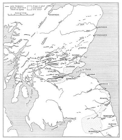
FIG. 1. Sketch-map showing distribution of quartz-dolerite and tholeiite dikes and associated sills.
