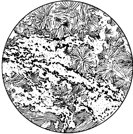
FIG. 1. Greenstone-hornfels, Zawn a Bal. Green hornblende, plagioclase, and streams of ilmenite.
