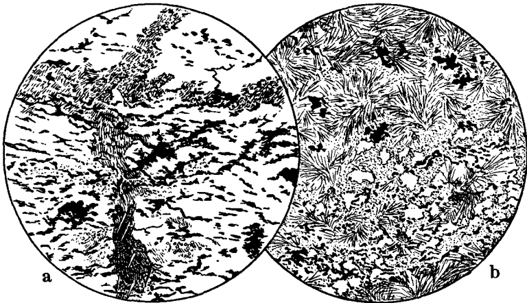
FIG. 3 a . Anthophyllite-cordierite-hornfels, Carn Kenidjack. Cordierite forms the colourless groundwork in the form of coarse-grained crystals through which pass streams of ilmenite. These are separated by threads of biotite with a crystal of anthophyllite at the bottom of the figure.
