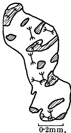
FIG. 2. Inversion intergrowth of braided larnite in a melilite-rock, showing the grouping of the parts into three sets, each with the acute bisectrix normal to the section, but with the mean optic axial plane directions of the sets inclined at 60^\circ to one another. Only one of the triple sets is shown in full development.
