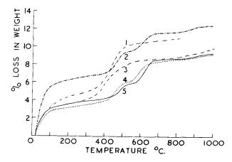
FIG. 4. Dehydration curves of illites.
