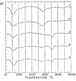
FIG. 3. Differential thermal analysis curves of illites.
