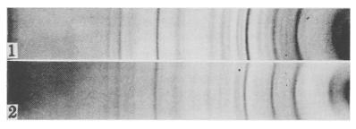
FIG. 1. Powder diffraction photographs of illites: 1, Ballater,  $< 1.4 \mu$ ; 2, Fithian, Illinois.
