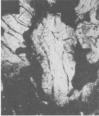
FIG. 1. Crystal of the phosphate phase in a basic open-hearth slag. Plane polarized light.
