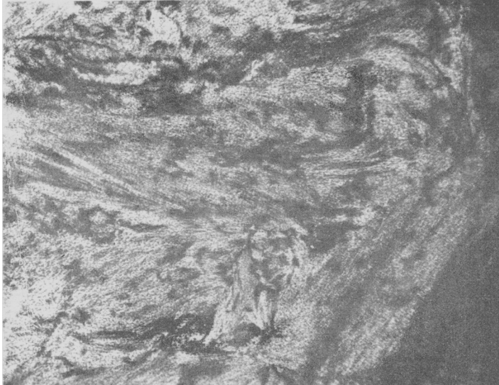
FIG. 1. Thin section of unaltered sillimanite rock. The whole of the field is occupied by uniformly fibrous sillimanite. Parallel nicols, \times 52 .
