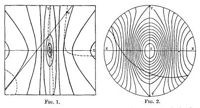
FIG. 1. The constant refractive index curves in the gnomonic projection for arbitrarily chosen values of  $\alpha$ ,  $\beta$ , and  $\gamma$ . The refractive index decreases from  $\gamma$  to  $\alpha$  along the X-axis, and from  $\gamma$  to  $\beta$  along the Y-axis. Point P represents the goniometer axis, and the line through P, a section of the crystal. The dotted curves are the vibration-direction curves (or extinction-direction curves) for the given position of P.
