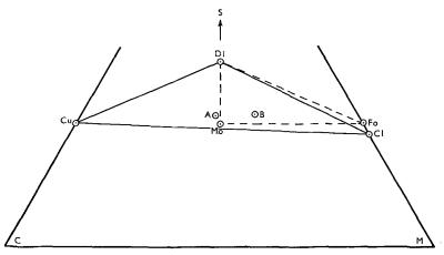
FIG. 14. Plot showing the compositions of the skarn zones diopside-cuspidineclinohumite (A) and diopside-monticellite-forsterite (B) in the system CaO-(Mg,Fe)O-SiO<sub>2</sub> (CMS). Cu cuspidine, Cl elinohumite, Mo monticellite, Fo forsterite.
