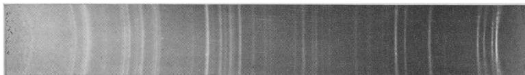
FIG. 1. X-ray powder photograph (cobalt radiation) of löllingite from Castle-an-Dinas mine, Cornwall. (High-angle end on the left.)
