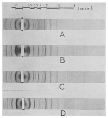
FIG. 2. X-ray diffraction diagrams of palygorskites: A, Bakkasetter, Shetland Isles,  $2-0.5 \mu$ ; B, Bakkasetter, Shetland Isles,  $< 0.5 \mu$ ; C, Cabrach, Aberdeenshire; D, Nawton, Yorkshire.
