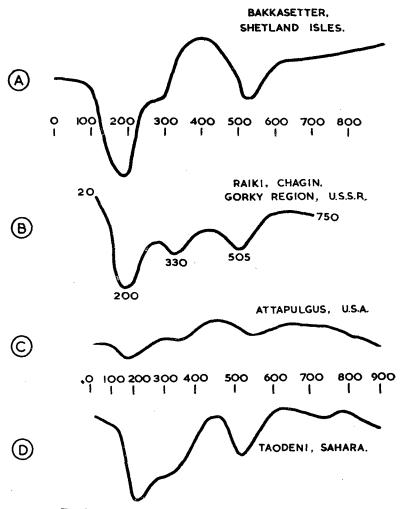
FIG. 3. Differential thermal analysis curves of palygorskites.
