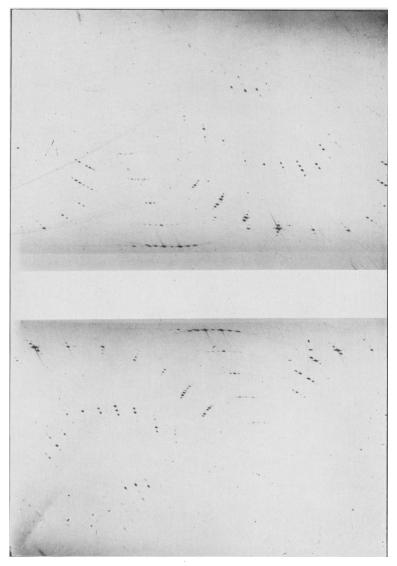
FIG. 2. Antigorite (Mikonui). Weissenberg (h0l) photograph. Ni filtered Cu- $K\alpha$  radiation.
