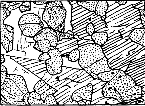
FIG. 2. Typical, coarse-grained picrite with large crystals of bytownite (toward left) and augite poikilitically enclosing olivines, the augite being moulded on the plagioclase. Interstitial analcite is not indicated. Sketched from a photograph. Scale: \times 18 .
