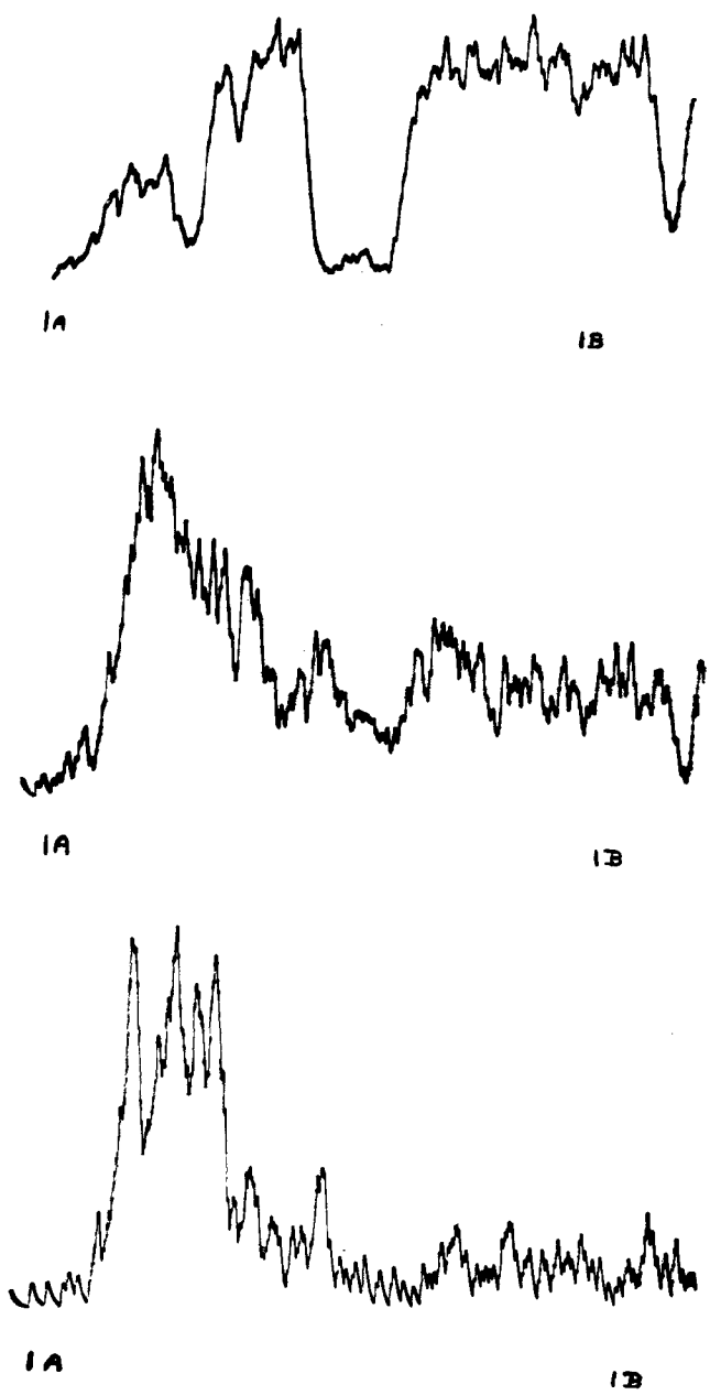
FIGS. 8 (top), 9 (middle), and 10 (bottom). X-ray traces showing the distribution of Ca, Sr, and Ba respectively across the traverse AB in fig. 7. The zero level of all three elements is given by the large trough corresponding to the siliceous inclusion. The unaltered pyrochlore contains approximately 10–15% Ca, a significant quantity of Sr and very little Ba. The altered portion is impoverished in Ca but shows considerable enrichment in Sr and Ba.
