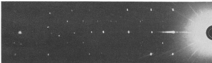
FIG. 1. Enlarged section of a c -axis photograph ( 15^\circ oscillation, \text{Cu-K}\alpha radiation) of an unheated hemi-hydrate crystal. Note intensity discrepancies for maxima on +1 and -1 layer lines and slightly variable \zeta values for spots on these layer lines.
