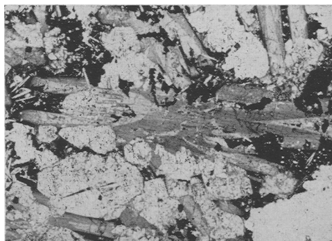
FIG. 5. Large augite crystal in ijolite from the Comores Islands. \times 5 . To be compared with the sketch in fig. 3C.
