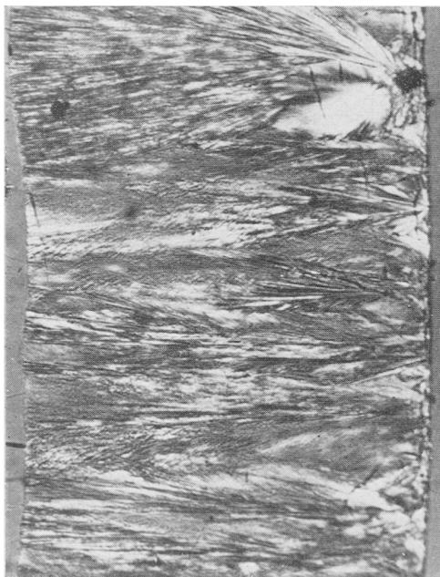
Fig. 1. Typical thin section of the crystalline surface layer of a heat-treated glass containing a small amount of chromium oxide. The crystals are an intimate mixture of wollastonite and anorthite. \times 300 .
