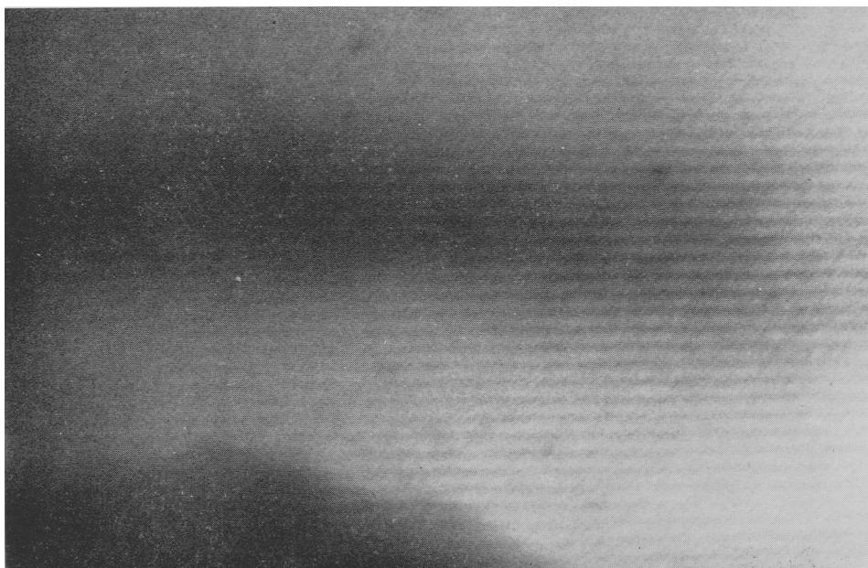
FIG. 5. Direct electron-optical resolution of the antiphase structure in an intermediate plagioclase feldspar. In this case the antiphase domain structure was resolved using the origin spectrum 000 and its associated f maxima. The specimen used had composition 70% mol. An, and was previously studied by Gay (1956, table 1, p. 25), where it is referred to as specimen 3. \times 530\ 000 .
