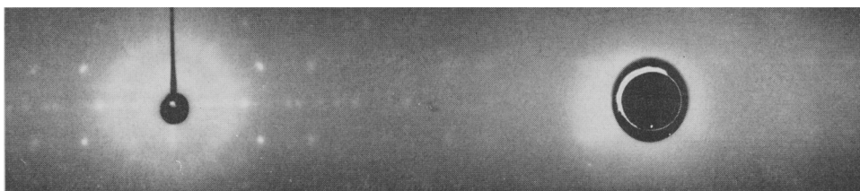
FIG. 6. Chip from intermediate zircon of density 4.18 \text{ gm cm}^{-3} , a axis vertical. Top . Laue photograph, c axis along beam, not filtered. Bottom . Rotation photograph, filtered.
