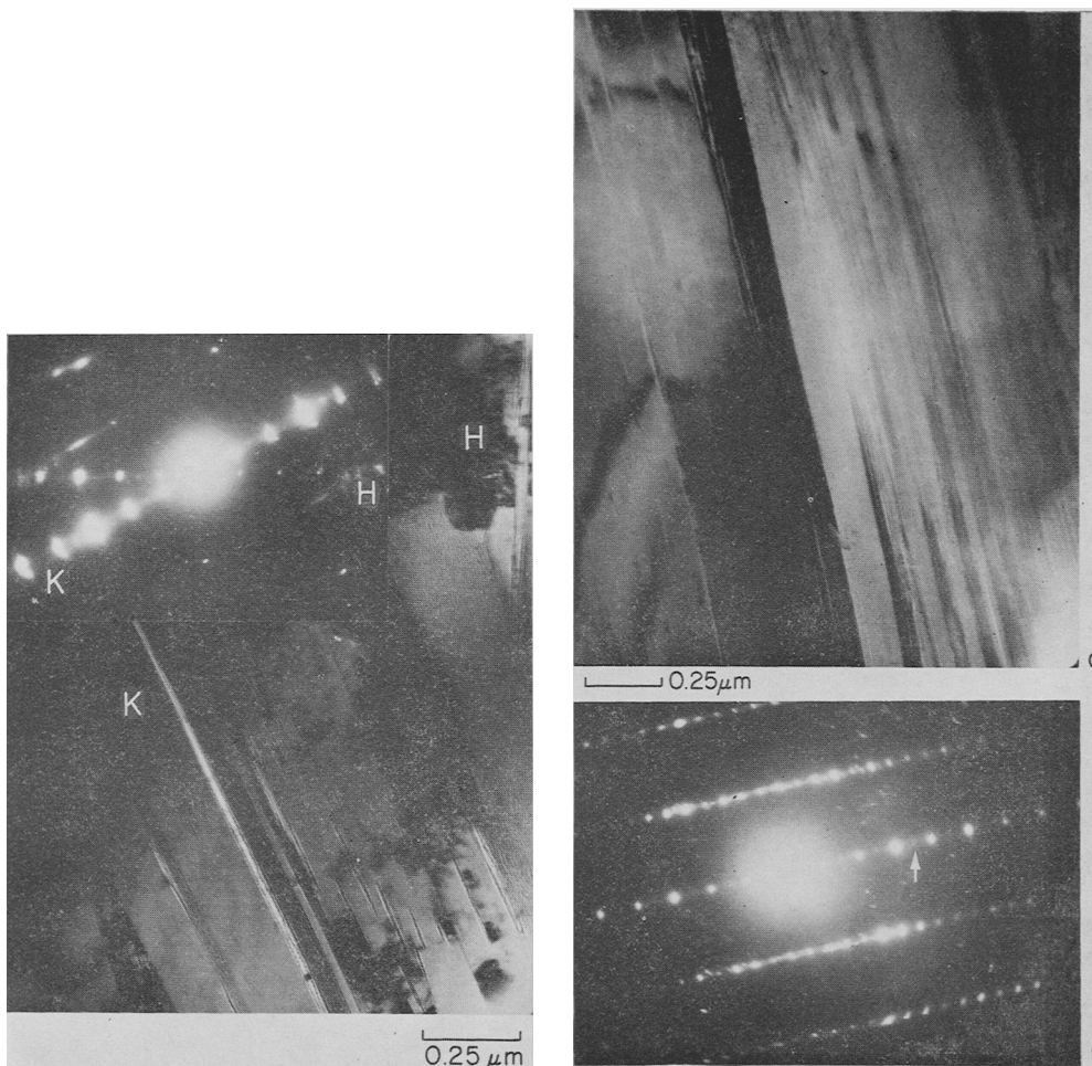
FIGS. 6 and 7: FIG. 6 (left). Transmission electron micrograph and selected-area diffraction pattern of two muscovite crystals in slate (Sample W22). Grain H shows weak superlattice spots 00l , odd l , in addition to the stronger normal spots. The larger grain—K—has a streaked pattern. FIG. 7 (right). Transmission electron micrograph (a) of a portion of large (approximately 7 \times 2 \mu\text{m} ) muscovite flake in siderite nodule (Sample CHH8) with selected-area diffraction pattern (b). Arrow points to diffraction spots for '007', a superlattice spot.
