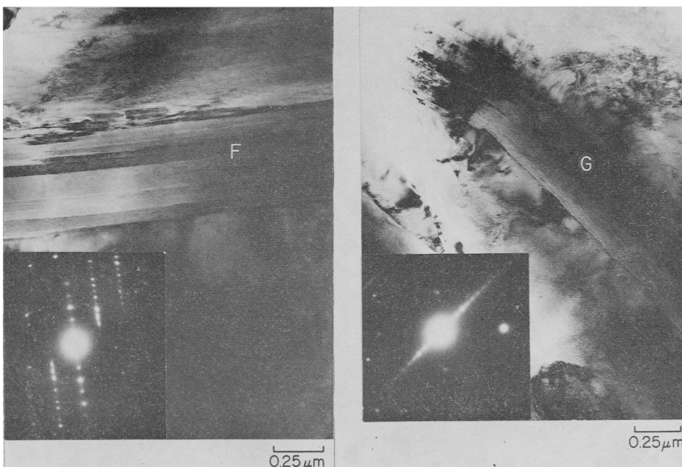
FIGS. 4 and 5: FIG. 4 (left). Transmission electron micrograph and diffraction pattern of muscovite flake embedded in siderite nodule (Sample CHH8). Pattern of 00l spots without streaking and restricted to spots for even l . FIG. 5 (right). Transmission electron micrograph and diffraction pattern of muscovite flake embedded in siderite nodule (Sample CHH8). The diffraction pattern shows a streak connecting the 00l spots of flake G. The material surrounding the flake is siderite.
