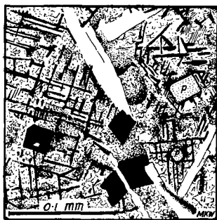
FIG. 4. Petrography of Type 2, represented by Specimen 1A, showing clear laths of plagioclase, sparse pyroxene (p), rutile and ilmenite rods, magnetite crystals, and dark-brown, almost opaque iron-rich patches which merge into the general matrix. This matrix is partly glassy, but poorly crystalline mica (top right) and microgranular patches of carbonate minerals (e.g. bottom right) can be distinguished with difficulty.
