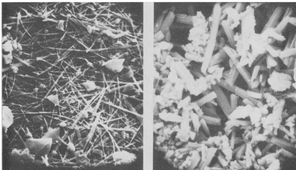
FIGS. 8 and 9: FIG. 8 (left). Scanning electron photomicrograph of fibrous todorokite. The irregular particles enmeshed in the fibres consist of kaolinite and unidentified crystalline and amorphous material. \times 7500 . FIG. 9 (right). Scanning electron photomicrograph of lathlike crystals of todorokite. No attempt was made to identify the small irregular particles dispersed over the todorokite laths. \times 10\ 000 .
