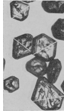
FIG. 1. A concentrate of tabular zircons showing an 'elongation' ratio of less than 1. The white lines drawn across some of the grains indicate directions of the [001] axes. Zoning and inclusions are apparent. Plane-polarized light, \times 60 approximately.
