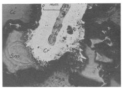
FIG. I. Photomicrograph to illustrate mineral association. Cc: calcite, Sm: smithsonite, Gt: goethite, Cr: coronadite.
