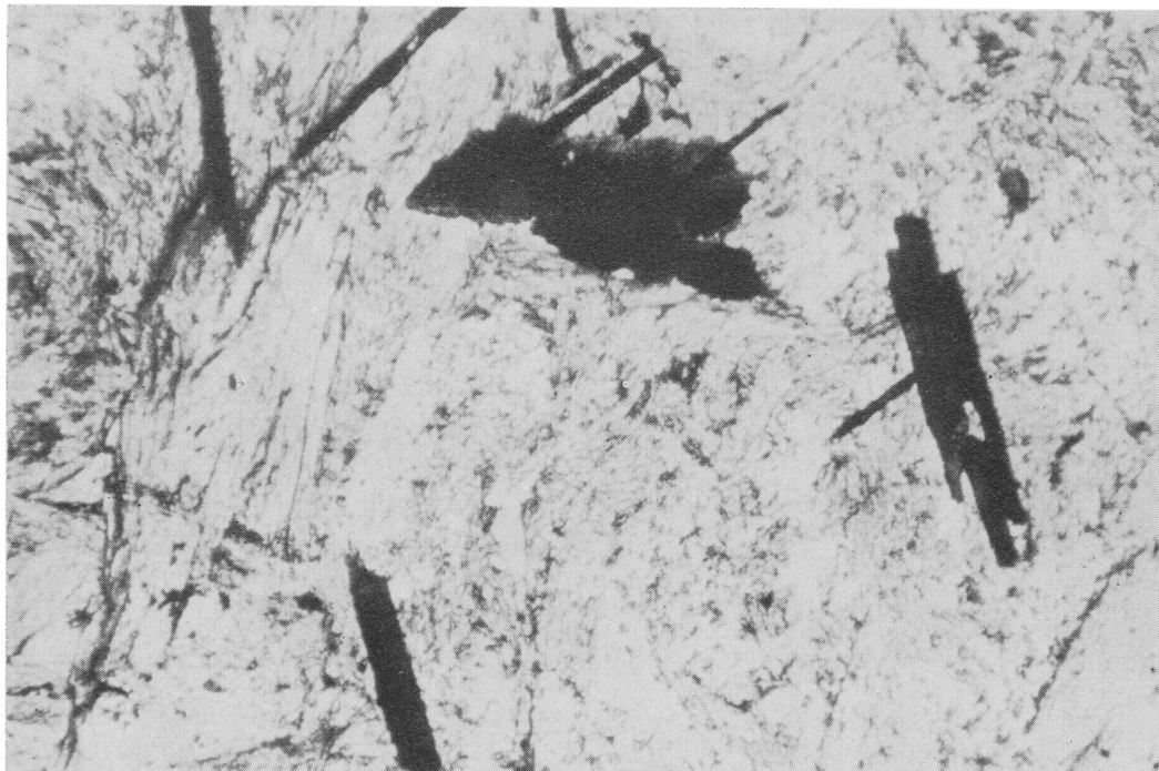
FIG. 2. Tabular crystals of högbomite (black) set within a matrix of sheridanite, a chlorite that has almost wholly replaced phlogopite. The large crystal on the right is 0.8 mm long. Sample 110.
