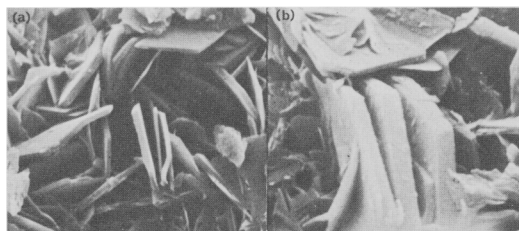
FIG. 1. Electron micrograph showing box-work of plate-like hexagonal crystals of motukoreaite forming cement in beach-rock. (a) x 10,000 (b) x 20,000.
