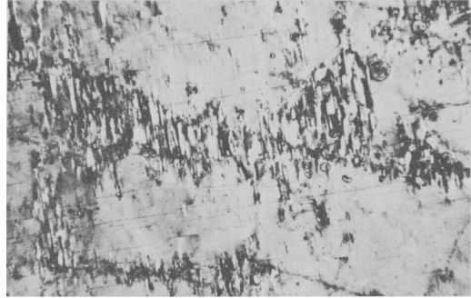
FIG. 3. Extreme contrast in coarseness of exsolution texture in a ternary alkali feldspar crystal, bulk \text{Ab}_{50}\text{Or}_{44}\text{An}_6 . Section cut approximately normal to x . The grey, apparently structureless areas are cryptoperthitic, transparent and show blue iridescence in hand specimen. The bands showing albite twinning are coarsely exsolved micropertthite, developed along cracks, which are white and turbid. The K-rich phase in these bands is inconspicuous because of the high contrast of the albite twins in the Na-rich phase, but microprobe analysis along the length of a coarsely exsolved area shows that the crystal has essentially constant bulk composition, and these bands are caused by coarsening, not replacement (crossed nicols).
