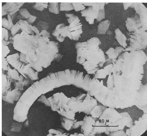
FIG. 1. Electron microscope photo of sasaite. Note the rhombic shape of the platelets and their accumulation along twisted axes.
