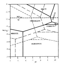
FIG. 2. Thermodynamic stability fields for the minerals. The bold lines indicate the extents of the fields calculated at  $a_{Ag}^{+} = 10^{-8} \text{ mol } dm^{-3}$  and  $a_{Cu}^{2+} = 10^{-8} \text{ mol } dm^{-3}$ . The Ag<sup>+</sup> - AgCl boundary at this  $a_{Ag}^{+}$  is denoted by short, firm dashes. How the fields are changed by increasing  $a_{Cu}^{2+}$  is shown for  $a_{Cu}^{2+} = 10^{-6}$  mol  $dm^{-3}$  (----) and  $a_{Cu}^{2+} = 10^{-4}$  mol  $dm^{-3}$
