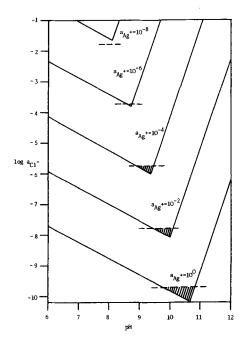
FIG 3. Areas of thermodynamic stability of boleite (hmtched) at  $a_{C_2}^2 r = 10^{-6} \text{ mol } dm^{-3} \text{ and } a_{A_R}$  as marked. Fields are bounded by others of pseudoboleite and cumengeite (firm lines), and the AgC1 precipitation limit (dashed line).
