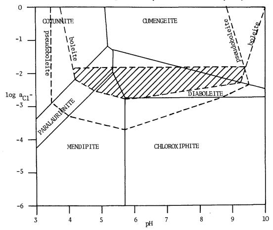
FIG. 1. Stability field diagram for the lead- and copper-chloride minerals. Boundaries are calculated for  $a_{Cu^{2+}}$  and  $a_{Ag^*}$  equal to  $10^{-6}$  and  $10^{-8}$  mol dm<sup>-3</sup> respectively. The boundaries for pseudoboleite and boleite are plotted separately as dashed lines. The hatched area indicates the range of conditions under which boleite may form metastably with respect to pseudoboleite. This field is bounded by the line above which chlorargyrite, AgCl, precipitates.
