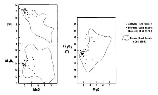
FIG. 3. MgO variation diagrams for tholeiitic lavas of western Kangerdlugssuaq. The solid line encloses the composition area for the Parana flood basalts (Cox, 1980) and crosses are selected data for Scoresby Sund basalts (Fawcett *et al.*, 1973).
