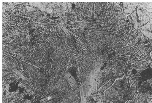
FIG. 1. Sample 173/33/K3/73 from De Beers Mine, Kimberley, South Africa. Numerous acicular or fibrous crystals of pectolite are the main constituent of the groundmass. Phlogopite ( p ), and opaque minerals including perovskite are associated with the pectolite. Olivine ( o ) can also be seen. Plane polarized light. Width of field = 0.6 mm.
