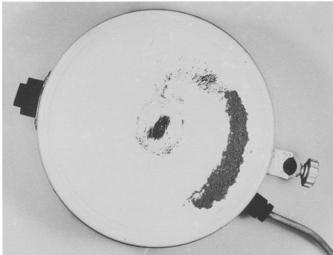
FIG. 1. Sample in process of separation; magnetic particles travel along a spiral path towards the centre of the rotating magnetic field.
