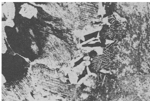
FIGS. 9 and 10. FIG. 9 (left). Photomicrograph of a lightly etched section of Pt_2FeCu showing decomposition along the grain margin with the appearance of the \gamma''_0 phase (16 × magnification). FIG. 10 (right). Photomicrograph of an etched section of Pt_2FeCu showing in greater detail the decomposition along grain margins to form the \gamma''_0 phase (160 × magnification).
