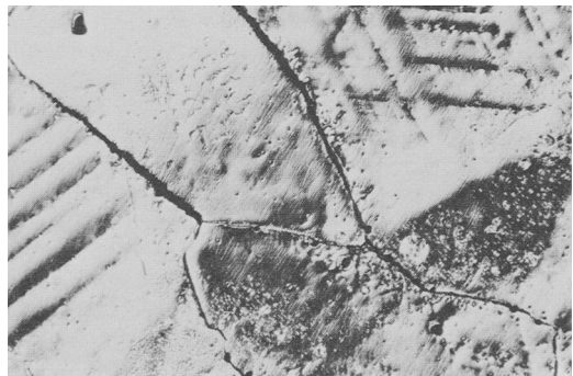
Fig. 6. Photomicrograph of thermally etched \text{Pt}_2\text{FeCu} showing grain boundary fractures ( 260\times magnification).
