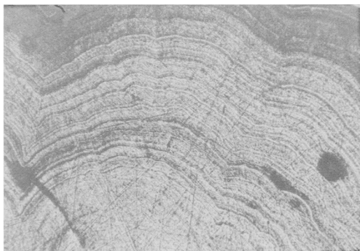
Fig. 2. Dark layers and white layers of the ranciéite colloform texture, reflected light, \times 500 .
