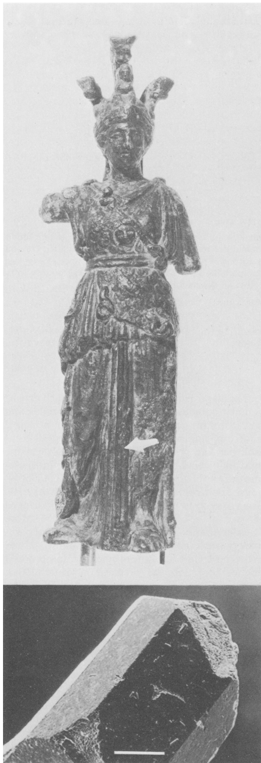
FIGS. 7 and 8. FIG. 7 (top). Statuette of Minerva (height 0.10 m). The arrow indicates the area of corrosion containing small pyroxene crystals. FIG. 8 (bottom). Pyroxene crystal observed in corrosion products on statuette of Minerva. SE image; operating voltage 25 kV. The scale bar represents 400 μm.
