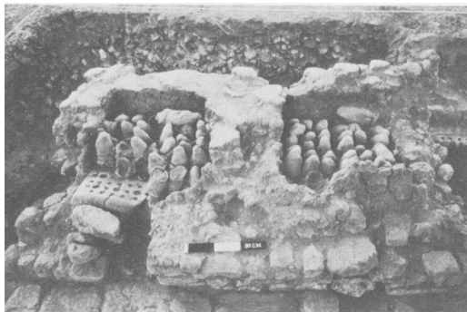
FIG. 9. Excavated zinc smelting furnaces at Zawar showing arrays of inverted ceramic retorts, supported by perforated plates (which divide the hot, upper chamber containing the retorts from the cool, condensation chamber below).
