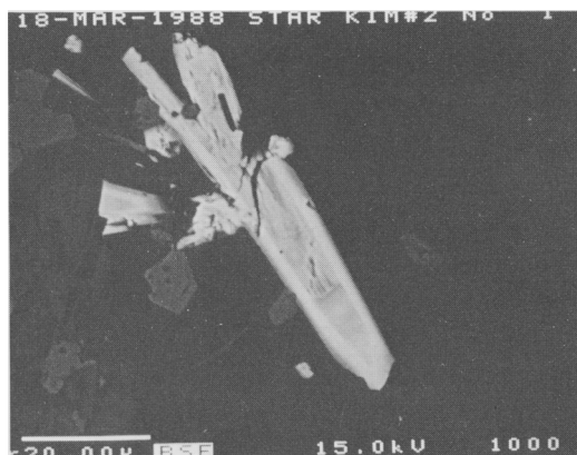
FIG. 1. Back scattered electron image of prismatic titanate. Compositions 3 and 4 (Table 1) are of the core and mantle respectively.
