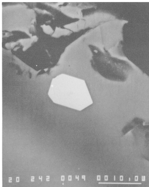
Fig. 1. Back-scattered electron image of (\text{Re},\text{Mo})_2\text{S}_3 crystal hosted by pyrrhotite.
