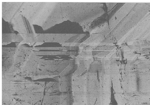
FIGS. 3 and 4. FIG. 3 (left). Type 2 banded sphalerite. The episodic nature of mineralisation is apparent with numerous discontinuities developed sub-parallel to banding. PPL Transmitted light. Field of view \sim 560 \mu\text{m} . FIG. 4 (right). Type 2 banded sphalerite showing textural modifications due to complex sector zoning and growth twinning. PPL Transmitted light. Field of view \sim 890 \mu\text{m} .
