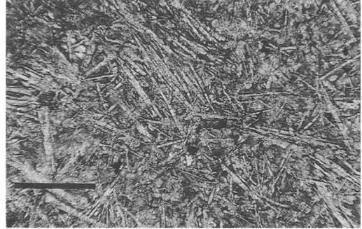
FIGS 1 AND 2. FIG. 1 ( left ). Photomicrograph of romanèchite aggregate. PPL, scale bar is 1 mm. FIG. 2 ( right ). Acicular and tabular calcite aggregates in BD83. PPL, scale bar is 0.5 mm.
