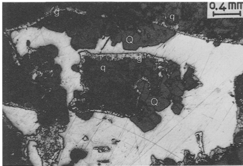
Fig. 5. Branch of tree-like bismuth-gersdorffite dendrites showing concentric gersdorffite (g) bands and infilling euhedral quartz (Q) and bismuth (white); fibrous-spherulitic quartz (q) radiates from dentate growth surface of gersdorffite. Reflected light.
