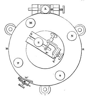
screws at the points Q, R, S, 38, 13, 25 millims. distant from the centre, for securing the crystal-holder to the instrument in a convenient position. This disk is capable of revolving round a pin the ends of which enter holes in the centres of the disk and graduated circle. A rectangular piece of metal T U, having each arm 95 millims. long, 30 millims. wide and 5
