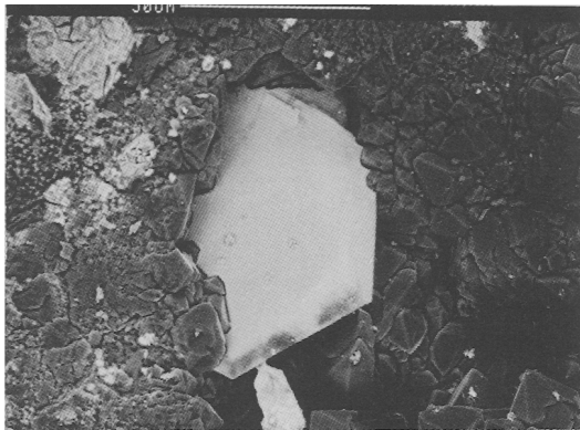
FIG. 1. Scanning electron photomicrograph of a leisingite crystal protruding from a small cavity. Matrix is quartz. (Scale bar: 50 \mu\text{m} ).
