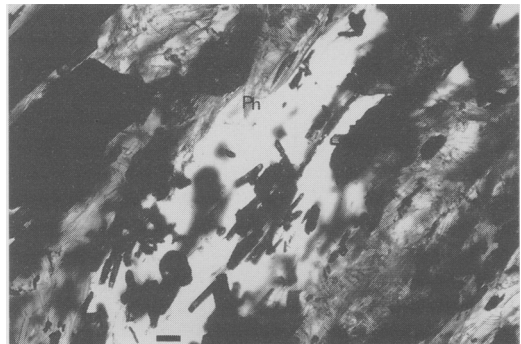
FIG. 1. Environment II. Plane polarized light. Scale bar = 40 \mu\text{m} . Elongated crystals of Sb-rich rutile occurring within the quartz-rich matrix but close to grains of piemontite (dark) associated with Mn-bearing phengite (Ph).
