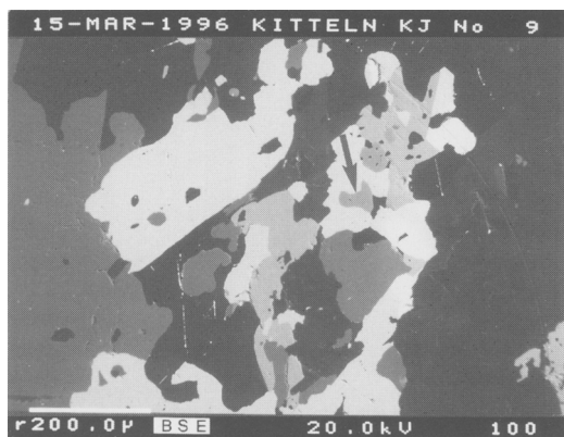
FIG. 2. Backscattered-electron image of manganostibite (white) in specimen #KG3, contiguous to katoptrite (light grey), tilasite (dark grey) and calcite (black). The arrow points to an intermediary grey phase, which is jacobsite. Scale bar (lower left corner) equals 200 \mu\text{m} .
