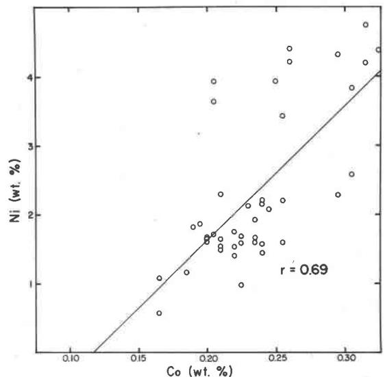
Fig. 3. Nickel and cobalt contents of 32 grains of low-Ni and 11 grains of high-Ni suessite from the North Haig ureilite as determined by electron microprobe analysis. Symbols as in Fig. 2.
