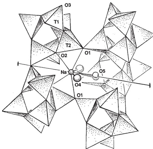
FIGURE 2. View of the crystal structure of tetranatrolite showing the location of the sodium atoms and the O4 and O5 water molecules within the Si-Al-O framework. A twofold symmetry axis, passing through O1 and Na, is shown.
