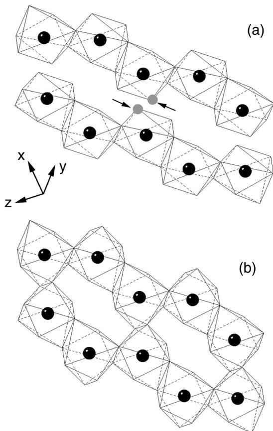
FIGURE 6. CaO7 polyhedra at room pressure (a) and above 5.8 GPa (b). The arrows indicate the oxygen atom which at high pressure connects to the neighboring chain and thus helps to form sheets parallel to  $(\bar{1}11)$ .
