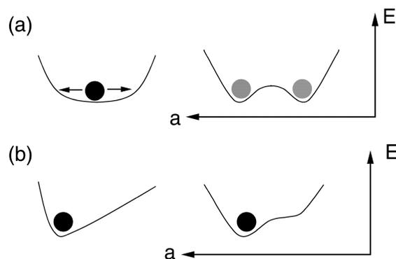
FIGURE 8. Schematic sketch of possible potential-energy curves of the Ca atom parallel  $[100]$  in the monoclinic (a) and triclinic (b) phase. Note that the large displacement parameter parallel  $a$  at ambient conditions can be explained by either a dynamic or a static disorder expressing either a flat potential well or a multiple-minima energy curve.
