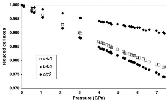
FIGURE 3. Reduced cell axes of malayaite as a function of pressure.
