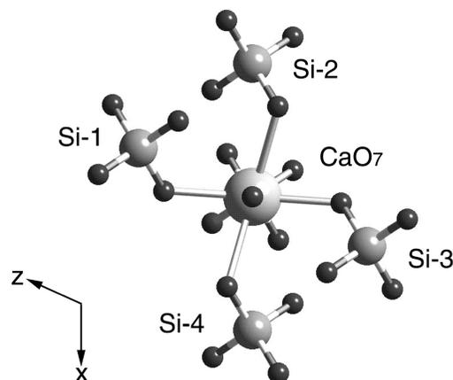
FIGURE 7. Sketch of the polyhedral environment of the Ca atom in the a-c plane. The Si-labels refer to the numbers in Table 7.
