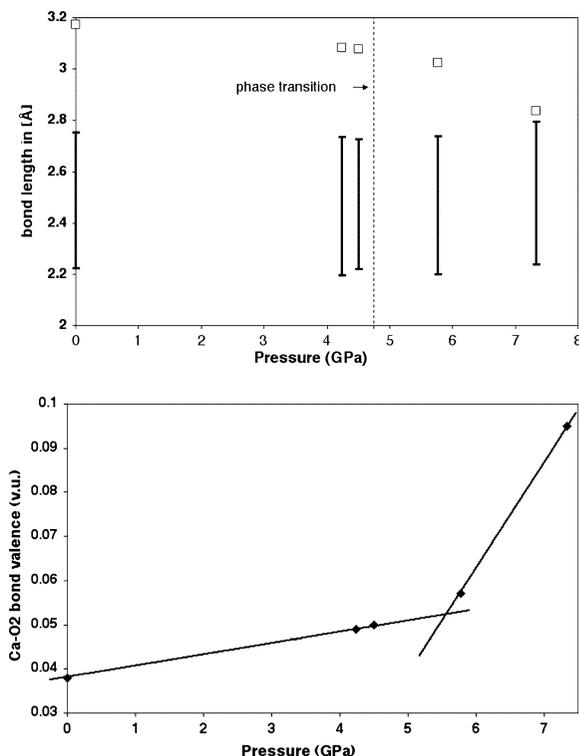
FIGURE 5. (a) Range of Ca-O bonds for  $\text{CaO}_7$  polyhedra (bars) compared with the approaching Ca-O2 bonds (open marks). Note that eightfold coordination is only achieved between 5.7 GPa and 7.3 GPa. (b) Plot of bond valences vs. pressure for Ca-O2. Note the sharp kink at  $\sim 5.8$  GPa, the same pressure where a change of slope is also noticed for the cell angles versus pressure. The lines are a guide to the eye.
