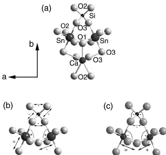
**FIGURE 1.** (a) Ball and stick model of a fragment of the malayaite structure. (b) Same fragment in the monoclinic phase at 4.505 GPa and (c) in the triclinic phase at 7.33 GPa.
