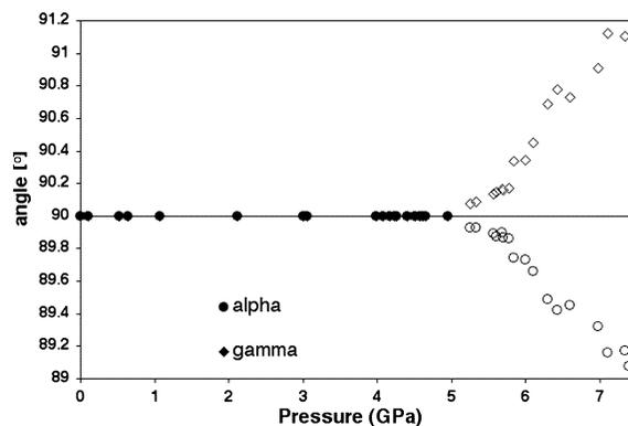
**FIGURE 2.** Evolution of the  $\alpha$  (circles) and  $\gamma$  angle (diamonds) as a function of pressure. The experimental uncertainties are smaller than the symbols. Full symbols mark the angle before the phase transition, open symbols denote the angle after the phase transition. Note the change of the slope at  $\sim 5.8$  GPa.
