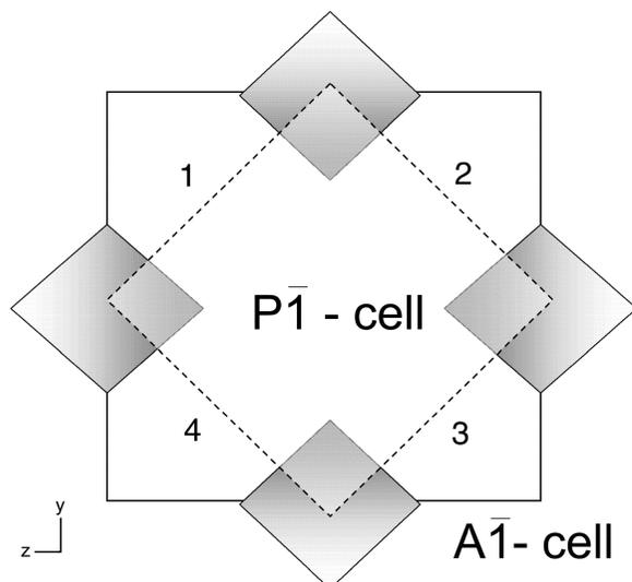
FIGURE 4. Schematic sketch of the  $A\bar{1}$  (solid line) and  $P\bar{1}$  (dashed line) setting for malayaite viewed along  $a$ . The diamonds represent the octahedral chains projected parallel to the  $a$  axis. The even-sided rhombohedral shape outlined by 4 neighboring chains becomes an uneven rhombus in the triclinic phase. The numbers denote the distances listed in Table 6.
