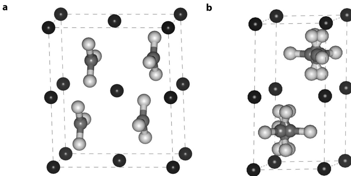
**FIGURE 1.** Crystal structures of vaterite. Scheme: light gray spheres are oxygen atoms, gray spheres are carbon atoms, and black spheres are calcium atoms. (a) Orthorhombic structure with space group  $Pbnm$  after Meyer (1959). (b) Hexagonal structure with space group  $P6_3/mmc$  after Kamhi (1963).
