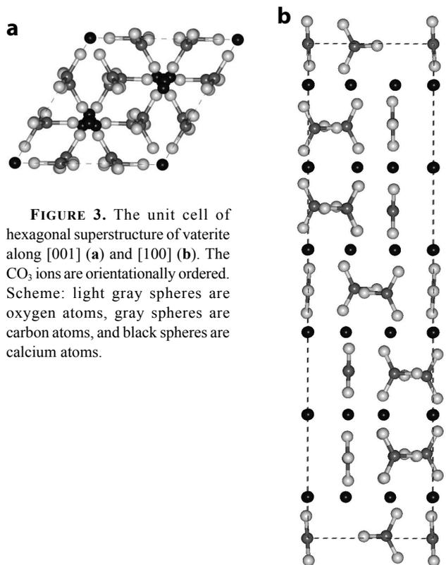
**FIGURE 3.** The unit cell of hexagonal superstructure of vaterite along [001] (a) and [100] (b). The CO<sub>3</sub> ions are orientationally ordered. Scheme: light gray spheres are oxygen atoms, gray spheres are carbon atoms, and black spheres are calcium atoms.
