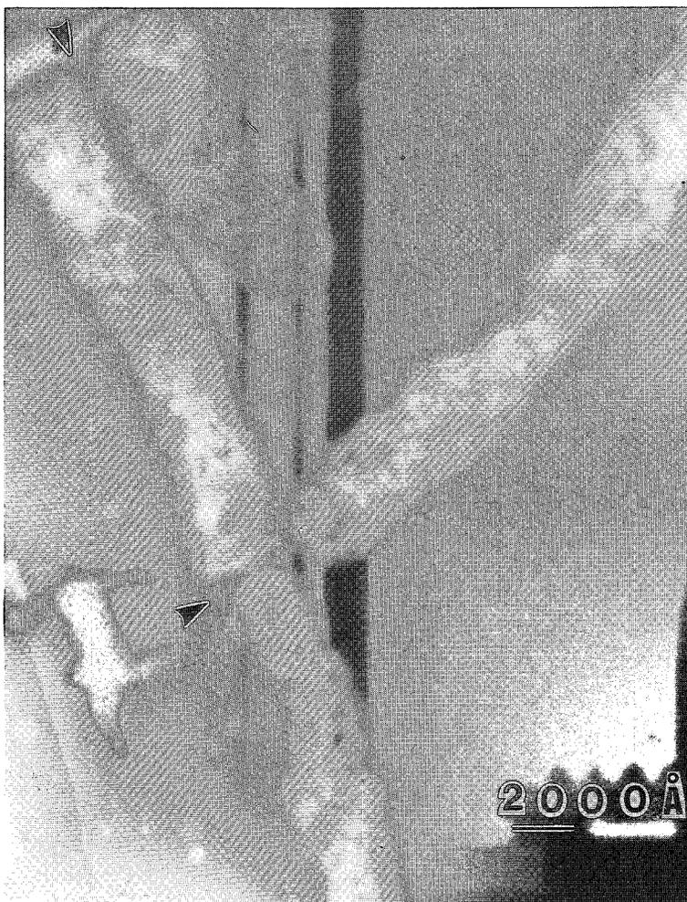
FIG. 5. Transmission electron micrograph of cultivated *T. thiooxidans* isolated from corroded sewer pipe at 30°C for 2 weeks using the AT medium. *T. thiooxidans* bacteria join at the arrow by a thin film.
