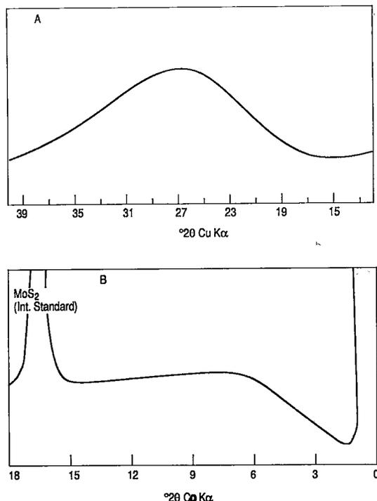
FIG. 1. X-ray-diffraction (XRD) patterns of the glass. A. Normal XRD. B. Low-angle XRD.
