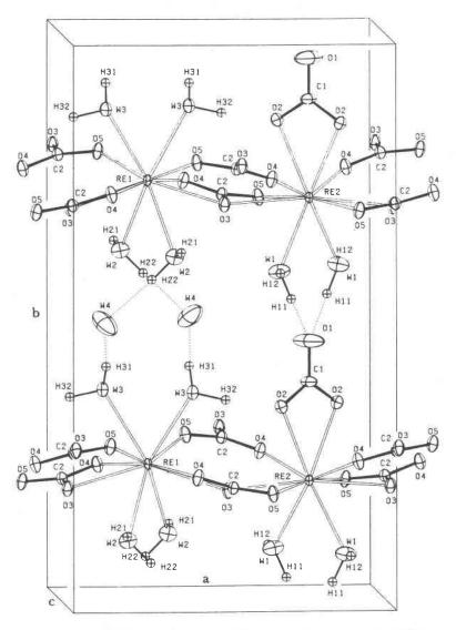
FIG. 2. ORTEP plot of the crystal structure of lanthanite showing the connection among adjacent layers of RE-O polyhedra.
